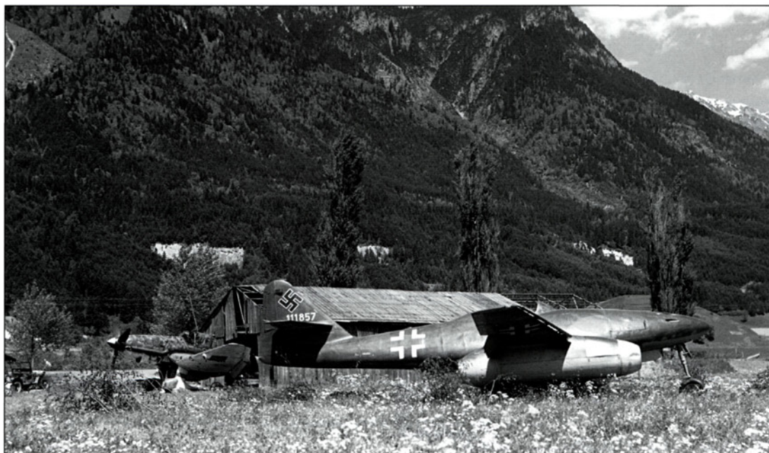
Seemingly incongruous amidst the spectacular mountain scenery towering above Hötting airfield is JV 44's Me 262 Wk-Nr. 111857. Bearing no tactical markings, the aircraft's distinguishing features are its prominent Werk Nummer and replacement cowlings around the engine intakes. Behind the Me 262 is Ju 87D-3 'E8+GL' of the night-harassment unit, NSG 9, complete with exhaust flame damper for nocturnal operations
