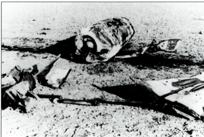
The extent of the crash can be seen from this photograph, showing one of the Jumo 004 engine units from Steinhoff's aircraft lying some way away from the main wreckage. Note the cowling panels to the right with the ports for the MK 108 cannon clearly visible
