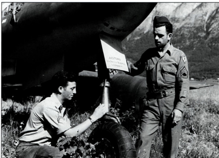
Mechanics of the US Ninth Air Force study the hydraulics on the nosewheel of an Me 262 of JV 44 at Innsbruck-Hötting. The stencilled marking on the nosewheel door reads 'ACHTUNG – Nicht am Bugrad Schleppen' (Attention! Do not tow by nosewheel). It was official practice to tow an Me 262 using a tow vehicle with cables fitted to lugs on the mainwheels
