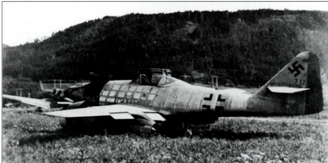
Me 262 Wk-Nr. 111712 was another aircraft to reach Innsbruck from Riem. This particular machine was distinctive by virtue of its bare metal finish, with much of its surfaces covered by filler paste
